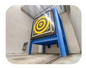
IRIS crash box system installed in the 20-meter-long custom designed test-pit. These will assure dampening of objects accidentally released during testing. Load absorption capacity is 5600 kJ which equates to an object mass of 300 kg travelling at 194 m/sec or 700km/h.
